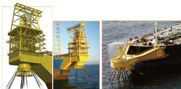
Abb. 14: Turret Mooring System zur Verankerung von FPSOs (Floating Production, Storage and Offloading Unit)
