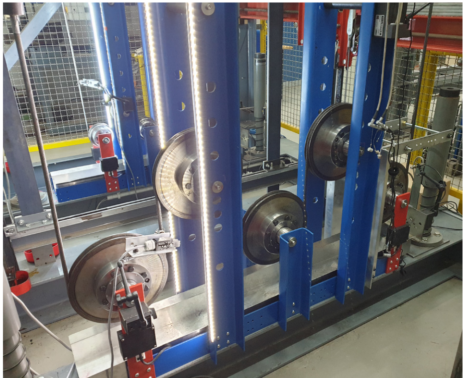
The five deflection pulleys connected in series in alternating direction
