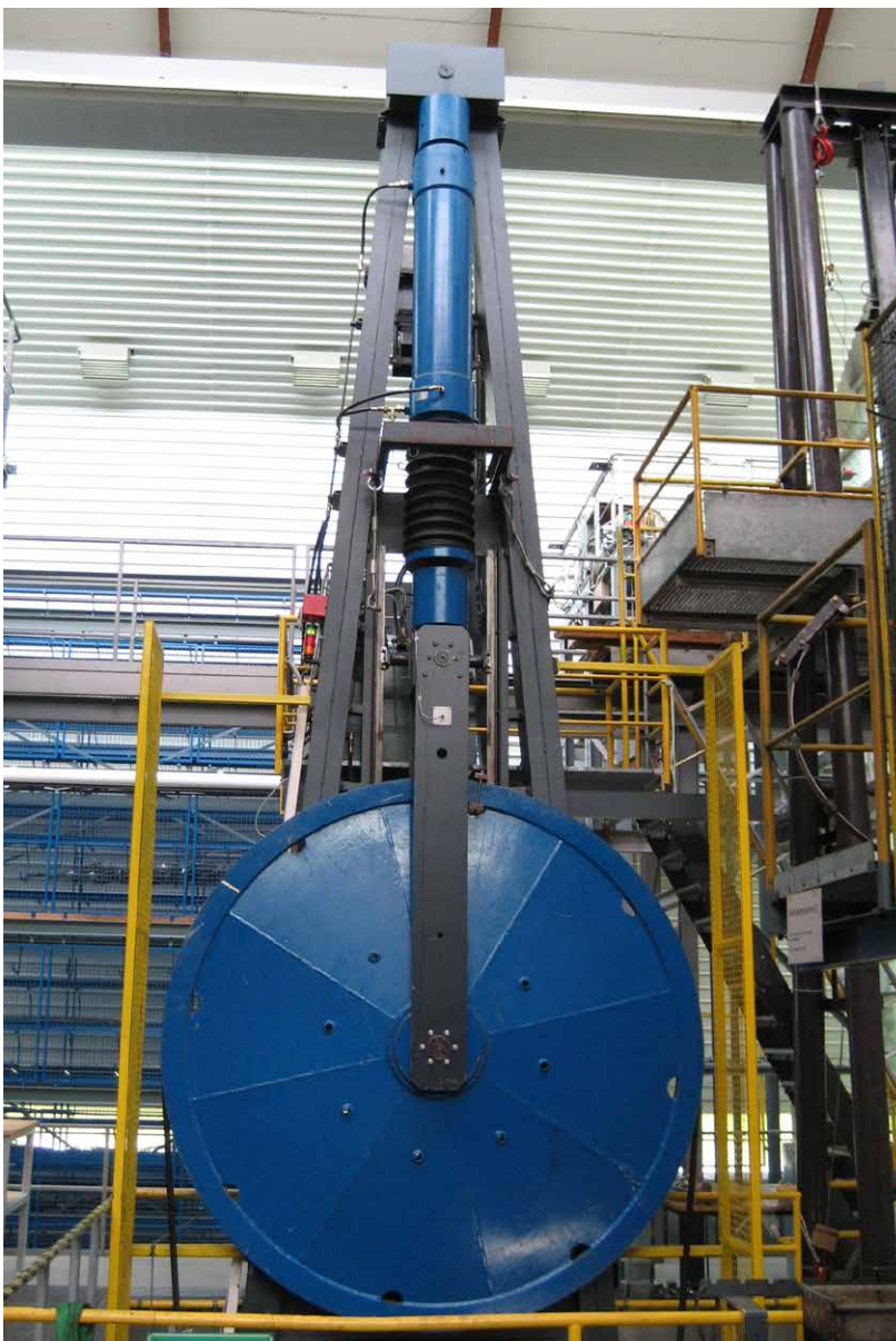
CBOS Test stand, max. test load 500 kN
