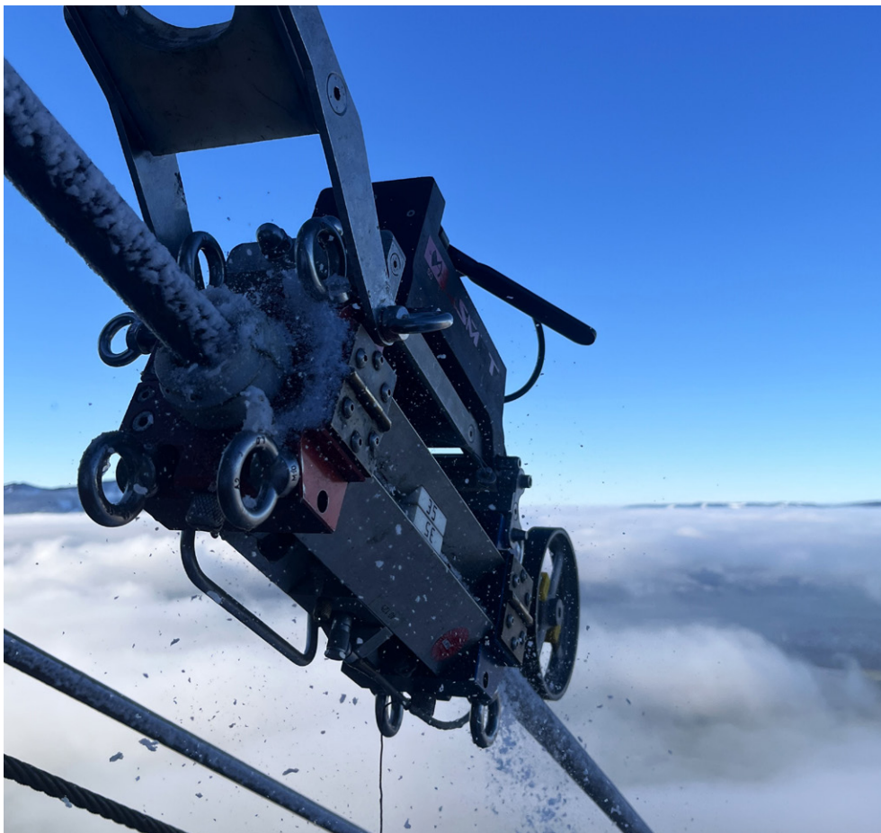
Magneto-inductive rope testing using SMRT test device in use
