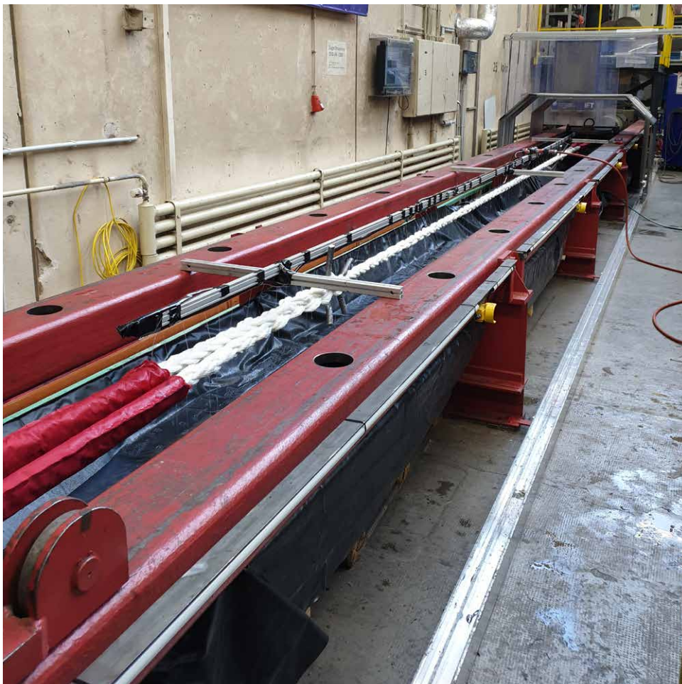
Tensile testing machine 2,500 kN
