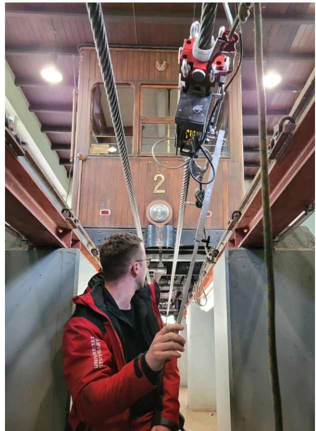
Magneto-inductive rope testing at Stuttgart Cable Car
