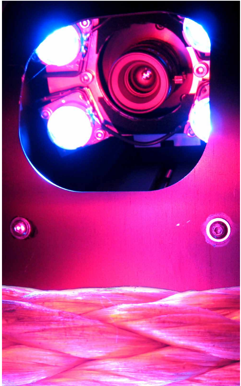
Digital visual surface inspection of Fiber Ropes
