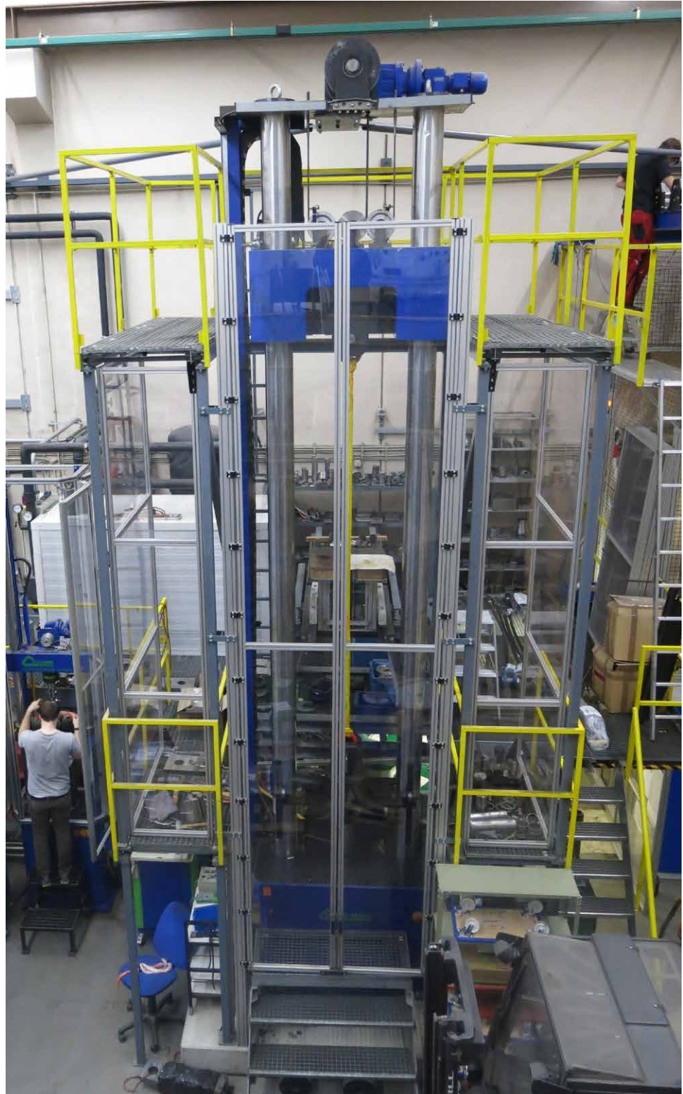
Testing machines for tensile and tension-tension testing
