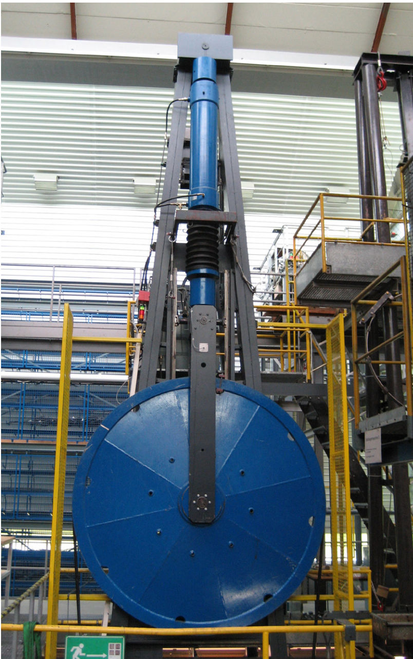
CBOS Test stand, max. test load 500 kN
