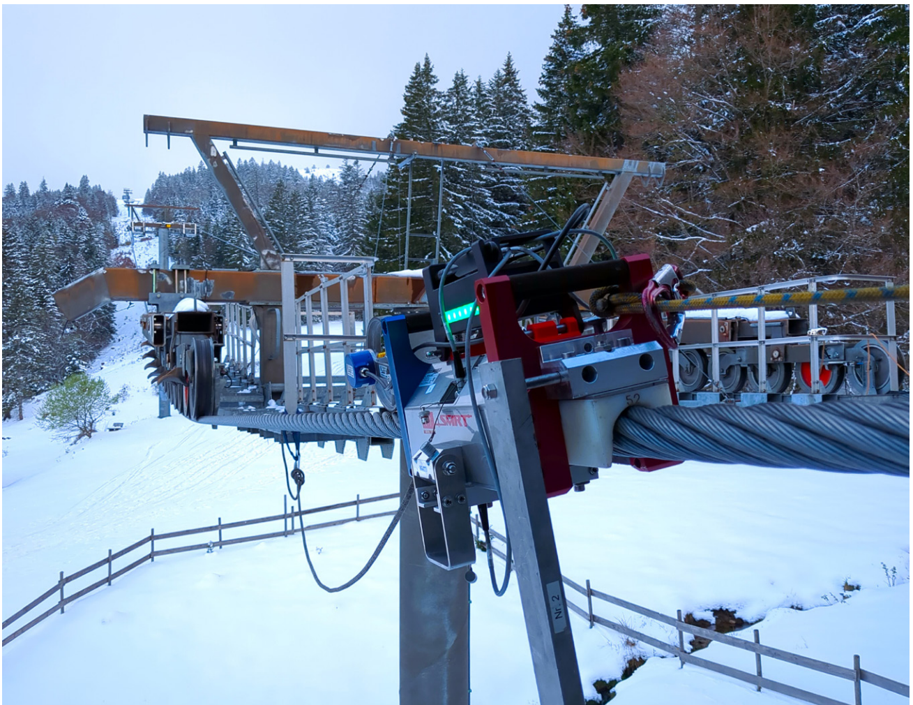
Magneto-inductive rope testing with the SMRT test device with measuring box
