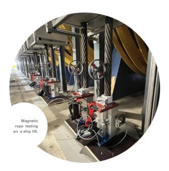
Magnetic rope testing in the field of passenger transportation technology is one of our core competencies. In addition to classic mountain ropeways, our test objects also include bridges, cranes, shaft hoisting systems and leisure facilities.
